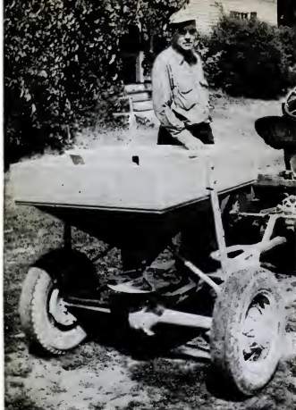
Model-A rear-axle assembly forms the chassis. Here, builder Howard Jenkins shows how the operator can ride on drawbar platform in field.
